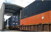
automated mechanical inspection while traveling at high speeds before train enters a yard
